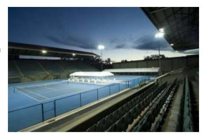
These supplemental flat glass luminaires provide the necessary vertical illumination for television coverage to CIE 169.
